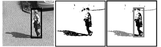
Figure 5: SNR Metric: (Left) Original with GT, (Middle) Detected Blobs (Right) Connected false positives
